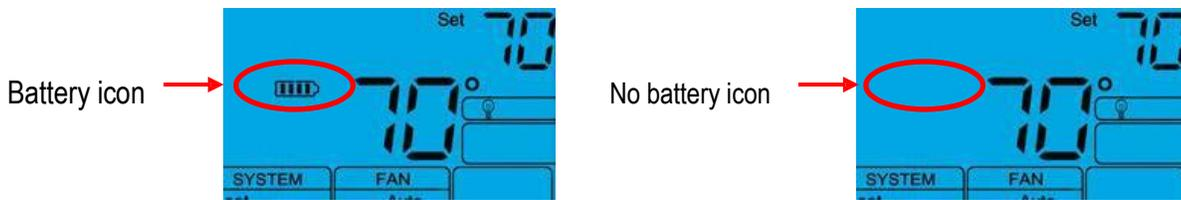
**Remedy:** Customers with a 1F8X-04XX thermostat that **does not** show a battery icon (🔋) on the thermostat screen should contact White-Rodgers for assistance with the corrective action or visit the White-Rodgers website. For affected thermostats, a packet will be sent which includes instructions on the corrective action.
